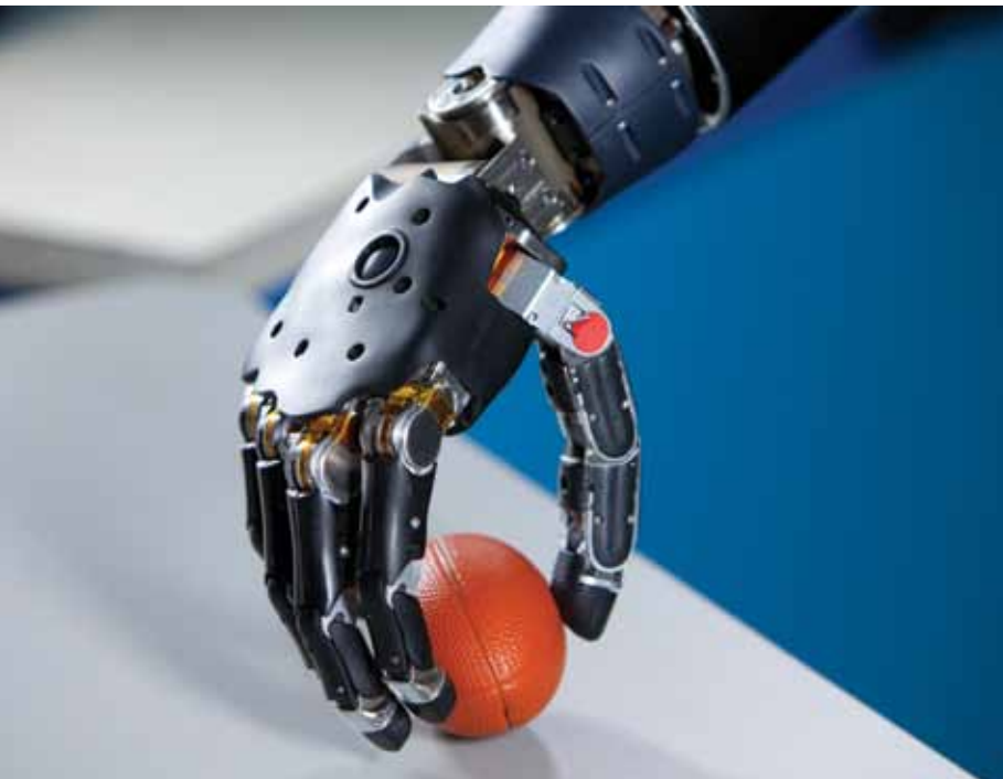
TOUCH THIS: A motorized tactor developed by Kinea (top left) mechanically stimulates an alternative body surface (top right) to “playback” the sensations picked up by fingertip sensors (bottom right) of a prosthetic hand. The Modular Prosthetic Limb (bottom left and page 41), developed by the Johns Hopkins Applied Physics Laboratory, uses the Kinea sensors in its fingertips.
